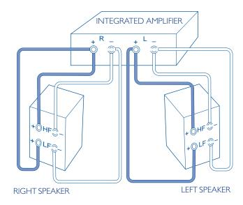
If you are using one pair of bi-wireable speakers and another pair that is not, you should connect your bi-wireable speakers as shown above, to just one set of the amplifier terminals. This leaves the second set of terminals to connect the non bi-wireable speakers to.
