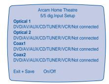
The DAVE module has 4 digital inputs (2 x optical, 2 x coaxial). Each of these can be allocated to one of 6 inputs DVD/AV/AUXI-CD/TUNER/VCR or Not Connected. Each digital input can only be allocated to one input e.g. if you chose Optical I to be for DVD the choices for Optical 2 are now only AV/AUX/CD/TUNER/VCR or not connected, etc. If you wish to re-allocate DVD to another input you must first change Optical I to another source, e.g. AUX, before you can allocate DVD to a different input.
